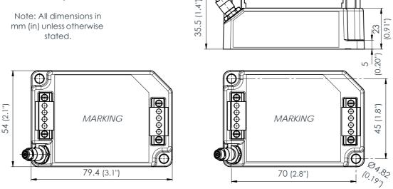
Side and end views with DIN-rail mounting adaptor (ordering option code G2)
