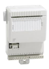
The DI801 is a 16 channel 24 V digital input module for the S800 I/O. This module has 16 digital inputs. The input voltage range is 18 to 30 volt d.c. and the input current is 6 mA at 24 V. The inputs are in one isolated group with sixteen channels and channel number sixteen can be used for voltage supervision input in the group. Every input channel consists of current limiting components, EMC protection components, input state indication LED and optical isolation barrier.
