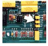
selected monitors, convenient firmware programming so that options can be changed easily and reliably in the field. The plug-in jumpers are simply repositioned on the monitor's circuit boards according to the legend on the monitor's protective side cover. The monitor's microprocessor continually checks the jumper locations and sets the monitor options accordingly.
