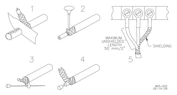
Figure 2-1. Preparation and Installation of Shielded Cables
