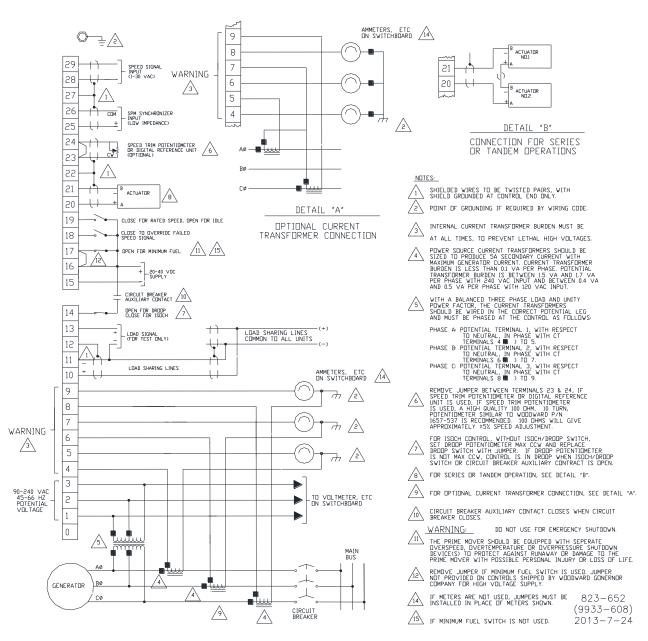
Figure 1-2a. Plant Wiring Diagram (low-voltage supply)
