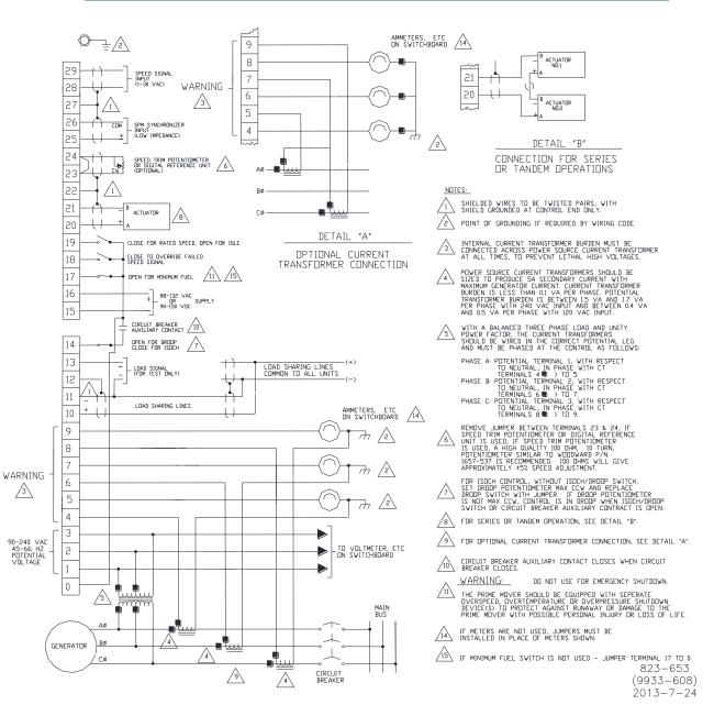
Figure 1-2b. Plant Wiring Diagram (high-voltage supply)
