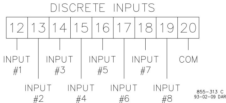
Figure 4-3. Discrete Input Connections
