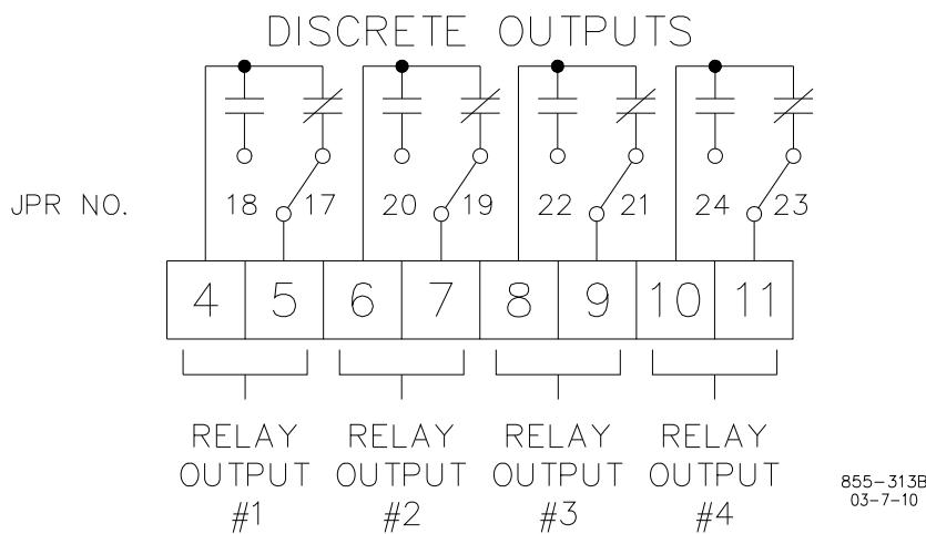
Figure 4-2. Relay Outputs
