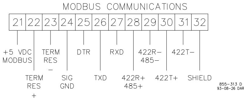
Figure 4-5. Modbus Connections
