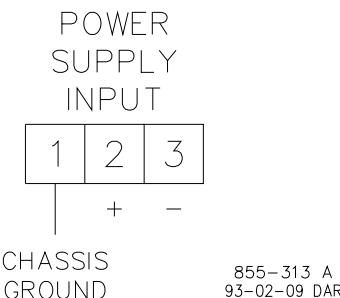
Figure 4-1. Power Supply Input
