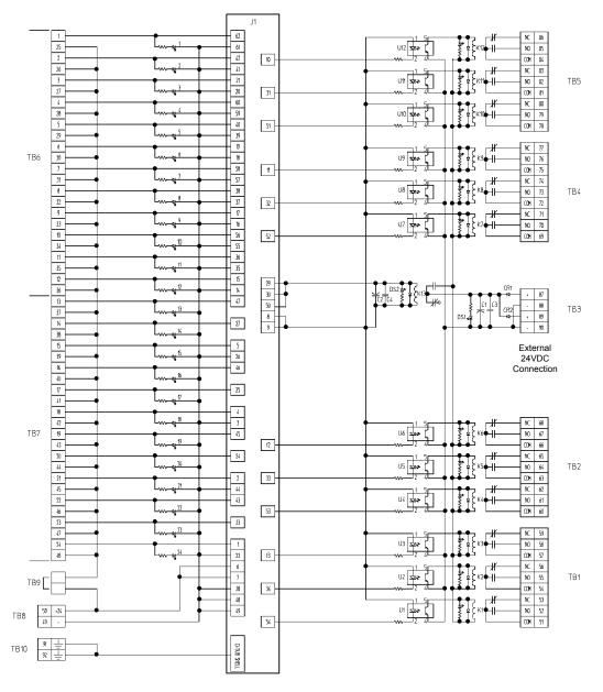
Figure 8-6—24/12 Discrete Module Schematic
