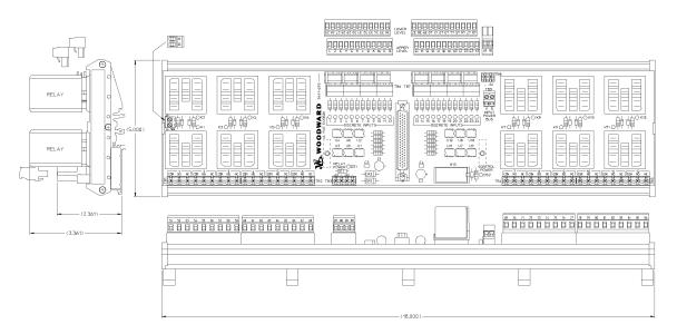
Figure 8-5—24/12 Discrete Module Outline Dimensions
