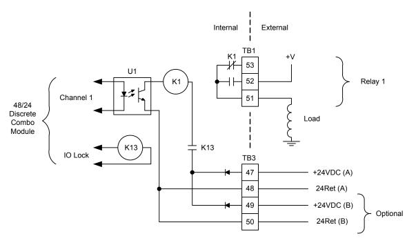
Figure 6-4—Relay Output Interface Wiring to a 24/12 Discrete FTM
