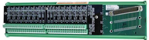
The 24/8 Analog FTM is used with the 24/8 Analog Modules (see Chapter 7 MicroNet module information and Appendix A for FTM part number). One MicroNet High Density Analog/Discrete cable is use to connect the FTM with the 24/8 Analog Module (see Appendix A for part numbers). There are twelve +24 Vdc connections available for sourcing 4-20 mA inputs. Each connection is protected with a 0.1 A fuse.
