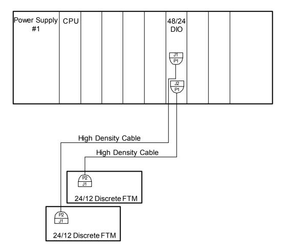
Figure 6-2—Configuration 2, Two 24/12 Discrete FTMs
