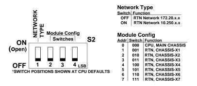
It is recommended to verify proper switch settings before installing the module in the system and when troubleshooting CPU-related issues.
