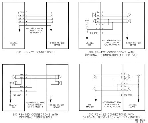
Figure 5-6—Termination and Cable Connection Examples
