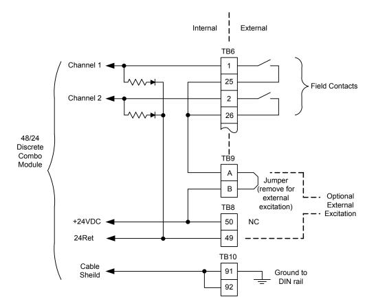
Figure 6-3—Discrete Input Interface Wiring to a 24/12 Discrete FTM
