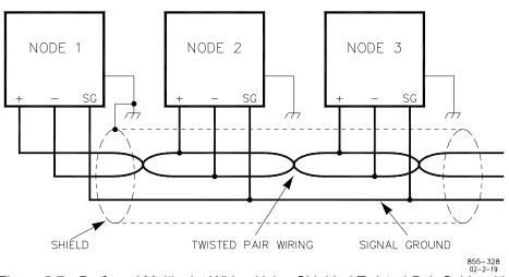
Figure 5-7—Preferred Multipoint Wiring Using Shielded Twisted-Pair Cable with a Separate Signal Ground Wire
