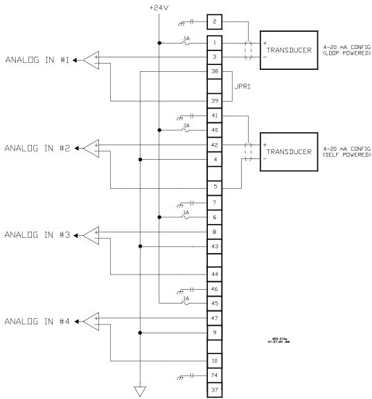
Figure 7-3—Analog Input Wiring for a 24/8 Analog FTM
