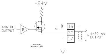
Figure 7-4—Analog Output Wiring for a 24/8 Analog FTM
