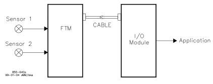
Figure 2-6—Redundant Sensors
