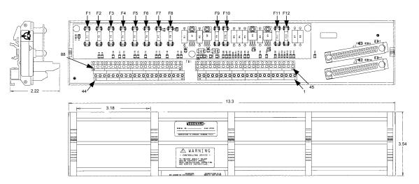
Figure 8-3—Analog Combo FTM Outline Dimensions
