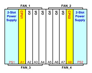
Figure 3-2—MicroNet Plus 8-Slot Chassis
