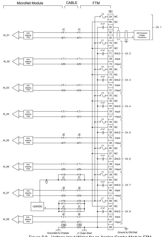
Figure 7-9—Voltage Input Wiring for an Analog Combo Module FTM
