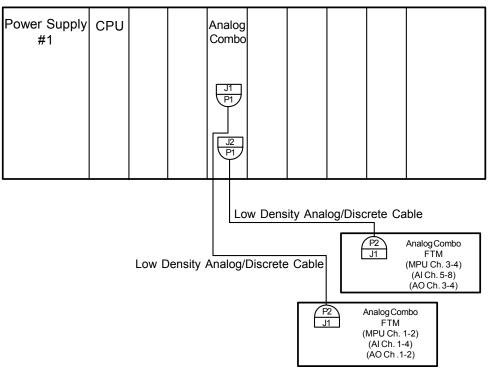
Figure 7-6—Simplex System Configuration Example
