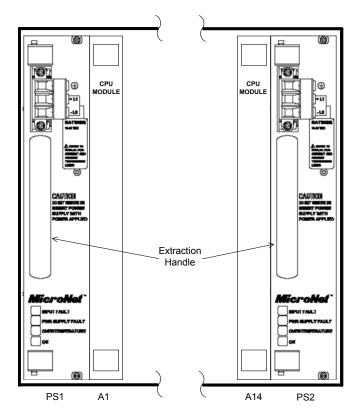
Figure 9-1—MicroNet Power Supply
