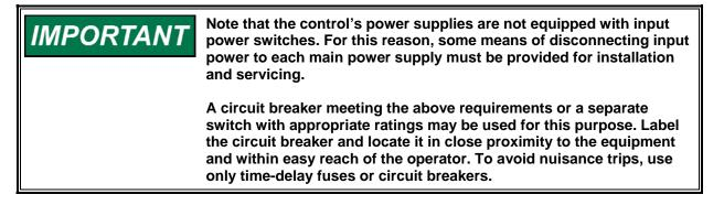
Branch circuit fuses, circuit breakers, and wiring must meet appropriate codes and authorities having jurisdiction for the specific country (CE, UL, etc). See Table 4-1 for maximum recommended fuse or breaker ratings. Do not connect more than one main power supply to any one fuse or circuit breaker. Use only the wire sizes specified in Table 4-1 which meet local code requirements. Time delay fuses or circuit breakers must be used to prevent nuisance trips.
