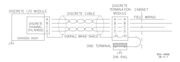
Figure 9-4—Discrete FTM Grounding Diagram Example
