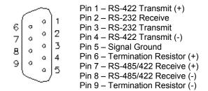
Figure 5-3—CPU Communications Port (DB9F)
